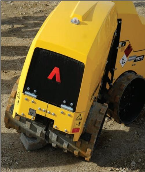
**Unique oscillating articulation joint** provides optimum traction and compaction on uneven surfaces. It also improves operational stability and reduces tip over risk.
