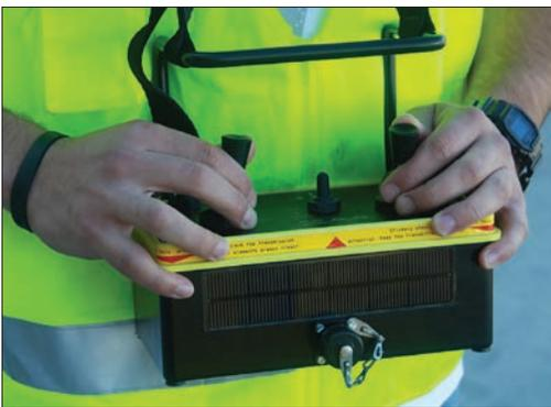
**Infrared (IR) control system** optimized for both operator safety and functionality. Requires visual contact with the machine for operation. Simplify fleet management by pairing transmitter to roller in seconds via cable connector. Blocks out signals from other machines on the job.
